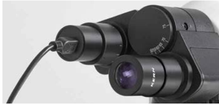
Eyepiece camera fixed into the tube
